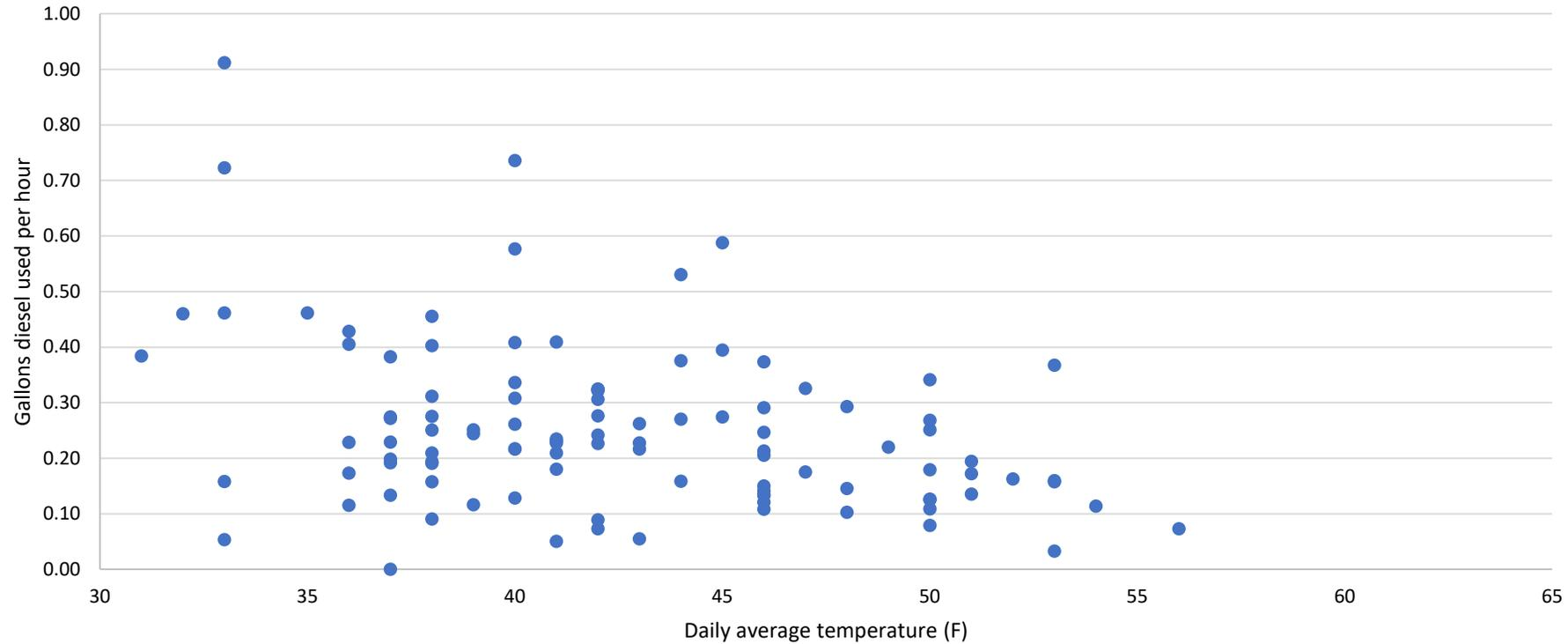
**Figure 12 notes:** Gallons of diesel used by the diesel heater per hour of operation was calculated for the fueling data provided by LTD. Operating hours for days where the bus was put into service but not fueled were added to the operating hours for the next day when the bus was fueled. Daily average temperature for the day the bus was fueled is used in the chart.
