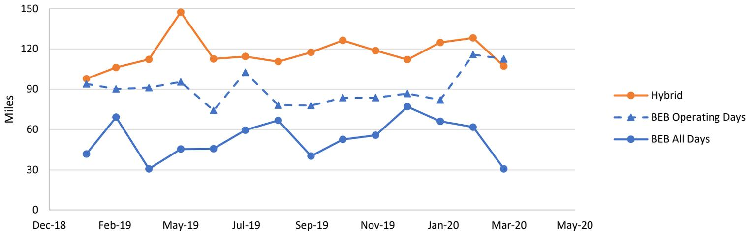
**Figure 2 notes:** The “Hybrid” and “BEB All Days” data series show the total monthly miles averaged over the total number of days per month and buses in the fleet, regardless of whether a bus was put into service. The “BEB Operating Days” series shows the total monthly BEB miles averaged over the days the bus was in service.
