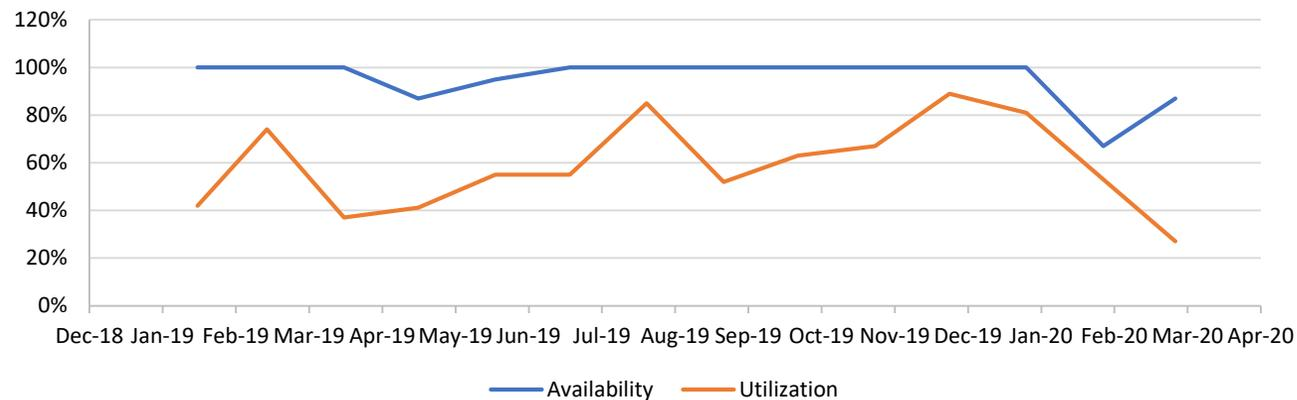
Figure 13 notes: Availability is the percentage of time a bus is categorized as "In Service" (Green), "Road Call" (Orange), or "Available, not in service" (Blue). Utilization is the percentage of time a bus is categorized as "In Service" (Green) or "Road Call" (Orange), and represents when a bus was put into service when it was available to do so.
