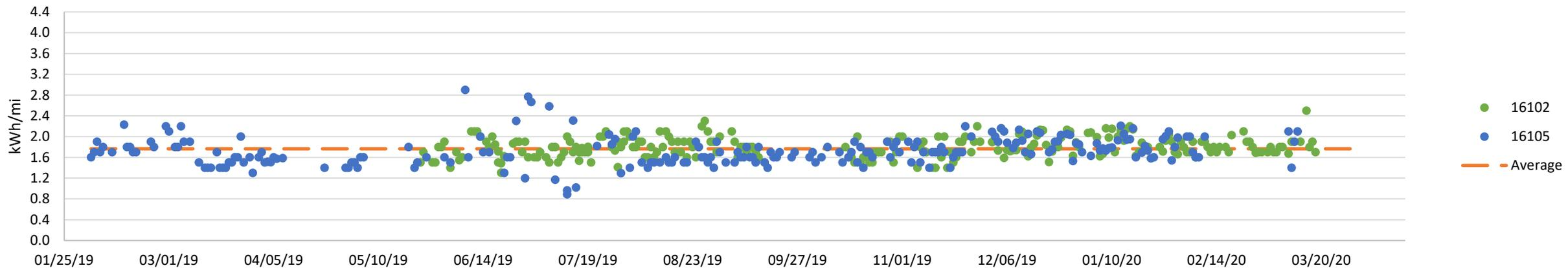
**Figure 5 notes:** Daily energy consumption (kWh/mi) by bus is shown, along with the overall average. HVAC consumption, driver style, and route conditions can impact energy efficiency.
