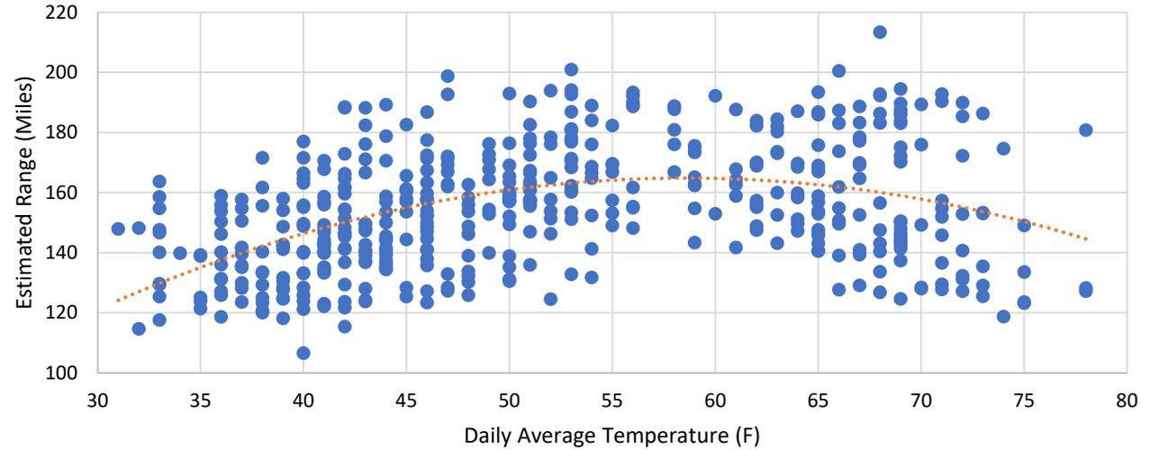
**Figure 10 notes:** Estimated vehicle range was calculated based off the %SOC per mile for each trip. The values represent the total estimated range if the bus is operated from 100% to 20% SOC.
