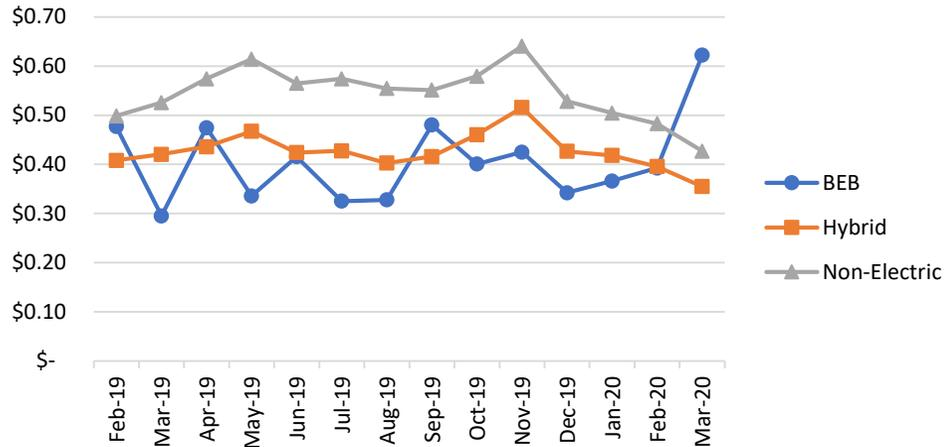
**Figure 3 notes:** Fuel costs per mile for the 16100 series BEB fleet, 16200 series hybrid fleet, and LTD's entire non-electric fleet are shown. Non-electric fleet fuel costs per mile fluctuate with changing diesel costs.
