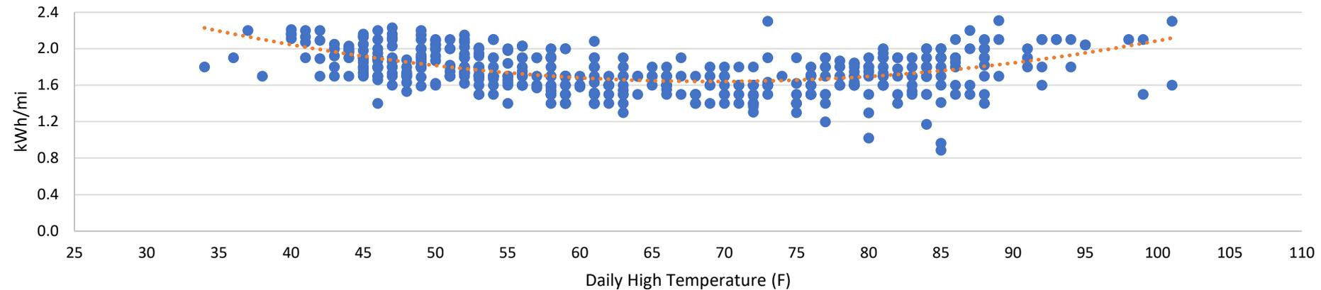
**Figure 8 notes:** Daily energy consumption (kWh/mi) by daily high temperature. In general, higher energy consumption is seen at very cold temperatures. Higher HVAC use in winter and summer months will most likely see the highest energy consumption.
