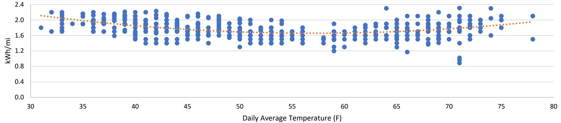
**Figure 7 notes:** Daily energy consumption (kWh/mi) by daily average temperature. In general, higher energy consumption is seen at very cold temperatures. Higher HVAC use in winter and summer months will most likely see the highest energy consumption.
