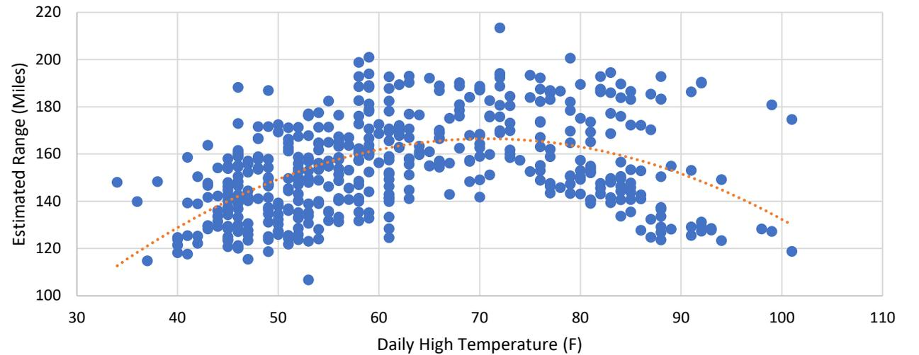
**Figure 11 notes:** Estimated vehicle range was calculated based off the %SOC per mile for each trip. The values represent the total estimated range if the bus is operated from 100% to 20% SOC.
