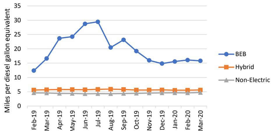
**Figure 4 notes:** Fuel economy for the 16100 series BEB fleet (miles per diesel gallon equivalent), 16200 series hybrid fleet (in miles per gallon), and non-electric fleet (in miles per gallon) are shown. BEB fuel economy increases in warmer months when the diesel heater is not utilized. Hybrid and non-electric fuel economies remain relatively constant.
